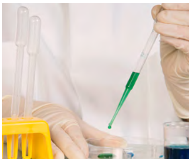
Figure 3. Disposable pipettes aid in accurate measuring of small volumes of liquids. It is important to use a new pipette for each chemical to avoid contamination.
