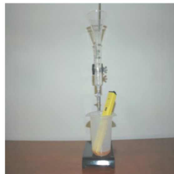
Figure 4. General set-up for titration and taking the pH reading.
