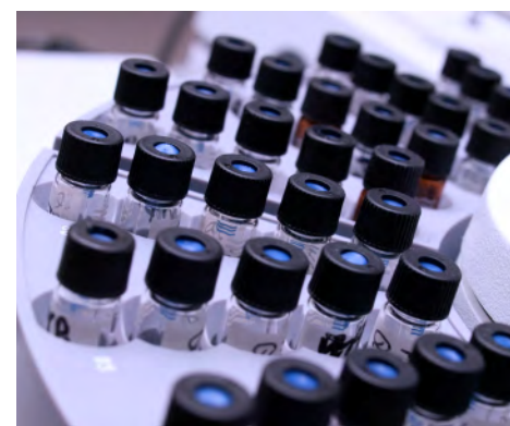
Figure 2. One type of chromatography used in laboratories is gas chromatography (GC). This is a picture of an GC autosampler.
