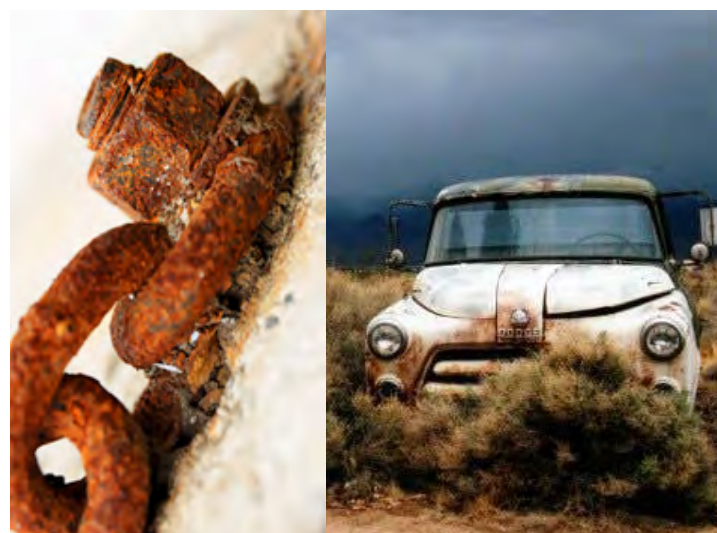
Figure 1. Rust is formed by the chemical reaction of iron and oxygen in the presence of water or air moisture.
