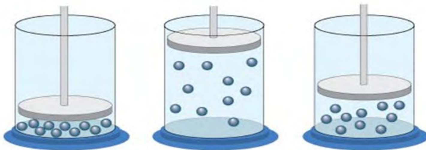
Figure 3. When the volume decrease, the pressure increases. Conversely, when the volume increases, the pressure decreases. This is what is known as an inverse relationship and is demonstrated in Boyle's Law (Figure 5).
