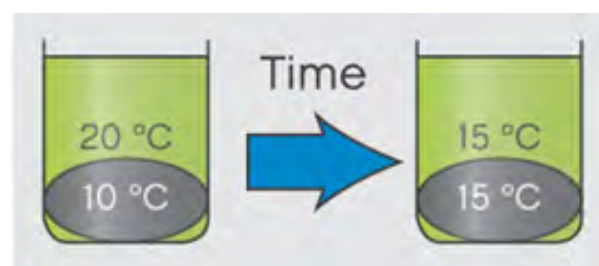
Figure 2. Given enough time the metal and the water will reach a state of thermal equilibrium and thus have the same temperature.
